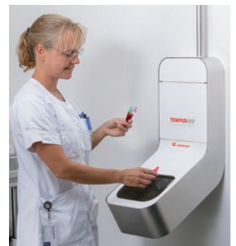
Samples are received in the Tempus600® Connection Module or the Receiving Tray in the laboratory.
