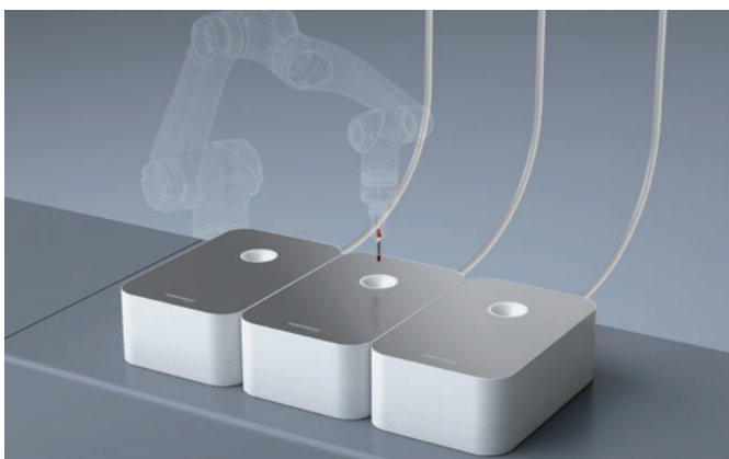
Samples are inserted individually by a robotic arm or other automated insertion.
