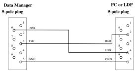
If the EDP system or the PC is operated with the RTS Signal (Request To Send):
